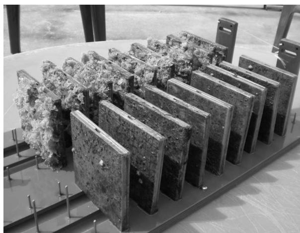
Figure 4. PVC panels after exposure for 4 weeks (15 July–12 August 2008). Non-aerated control panels are in the back row, aerated panels are in the front row.
